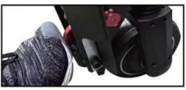
Check that the scooter looks to be ok Be sure that the valve is open and press on the red handle. Easiest way is to push rear wheel against the handlebar post to ease the pressure on the lock.
