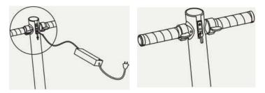
Always cover the USB charging port after charging. Charging must take place in an area children do not have access to. Avoid using other chargers as this may damage the battery and the device. Do not disassemble the charger if it is not working properly. Avoid charging indoors Always be present Do not charge at night Disconnect the charger immediately if you notice a strange odor or the charger is too hot. The e-scooter should be recharged a few times during the winter to preserve the battery.
